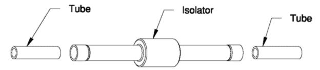
Solder or Braze tube into isolator tube ends.
