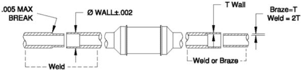
Braze or Weld tube into isolator tube ends.
