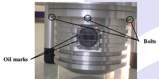
Figure 4-5 Oil sump of oil lubricated pump
